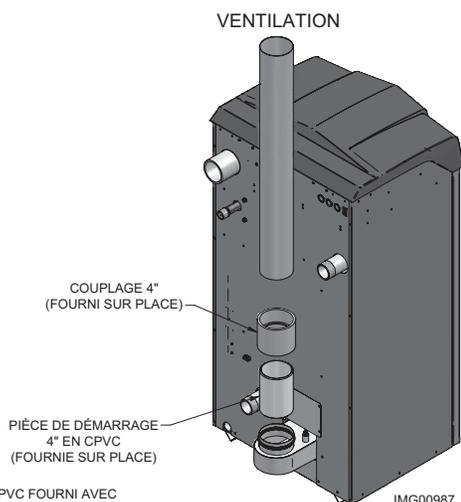
LE TUYAU de 4" EN CPVC FOURNI AVEC LE CHAUDIÈRE DOIT ÊTRE UTILISÉ POUR LE RACCORDEMENT DE LA VENTILATION
