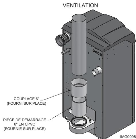
LE TUYAU de 6" EN CPVC FOURNI AVEC LE CHAUDIÈRE DOIT ÊTRE UTILISÉ POUR LE RACCORDEMENT DE LA VENTILATION
